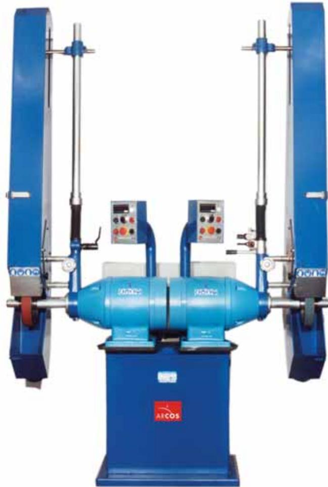
2TS/B 2 Heads Grinding Machine Unit with Electronic Speed Variation
